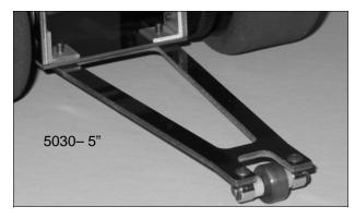
5320 ALUMINUM CLAMP HUB HOLDS THE GEAR AND A 2 BOLT 1/12 SCALE WHEEL. USE THE SAME FOR THE LEFT SIDE. SOME RACERS PREFER 1/12 WHEELS ANDTIRES SINCE THEY ARE A
