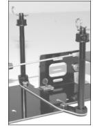
STEP 11 OPEN BAG 4. ATTACH THE 5581 GEAR TO THE 5312 HUB WITH TWO 3/8" LONG SCREWS. DO NOT OVERTIGHTEN!
